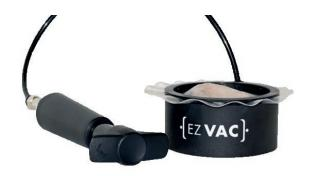
A simple-to-use vacuum forming device specifically designed to allow the manufacture of perfectly adapted, thin FiBERFORCE" reinforcements - every time. Through the use of a vacuum pump, a silicone membrane pulls down on the Splintvac mesh to precisely adapt the mesh to the model. The result is then inserted into a light-curing unit and quickly cured into its final shape.
